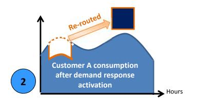
3<sup>rd</sup> party aggregator requests Customer A to reduce consumption while the BRP/supplier supplies electricity as forecasted. As a result:
